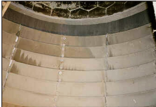
Typical wear regions on internals of separator
